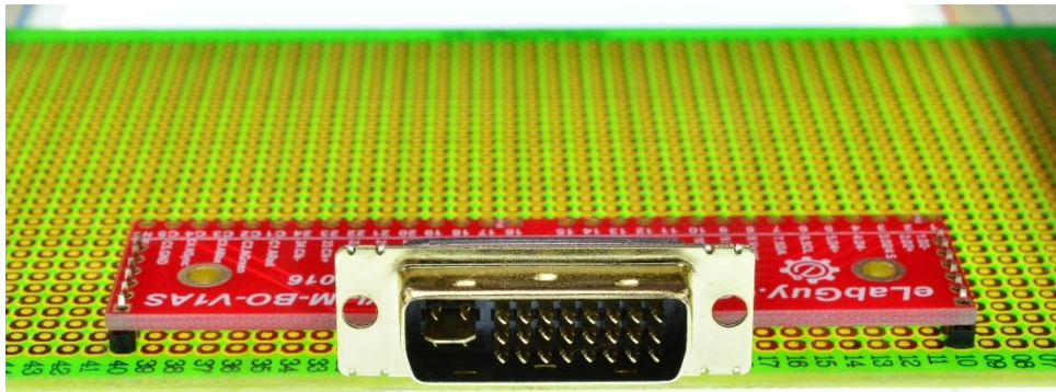
Figure 4: Solid Mounting on prototype PCB
